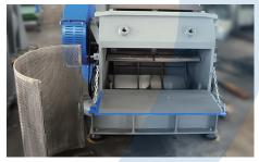
The redesigned base of the GSE 700 series makes the machine very sturdy, while maintaining the easy accessibility for maintenance and cleaning.
