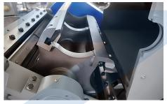
The GSE granulators are available with different rotor options to fit different applications, all rotors feature the V-cut technology creating a high quality regrind.
