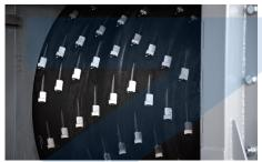
The ZRS shredders use very large diameter flat E-style rotors. The knives are fixed in special knife holders fitted in machined pockets.
