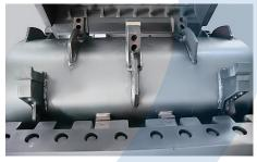
The combination of pre breakers and counter knives create a high impact powers resulting in a high degree of disintegration and high throughput rates.
